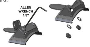
The Body Assembly must be removed to gain access to the CLAMP SCREW. Remove the two socket head screws as shown below. Be sure to remove the lock washer with the top screw along with the lock washer and flat washer with the bottom screw.
