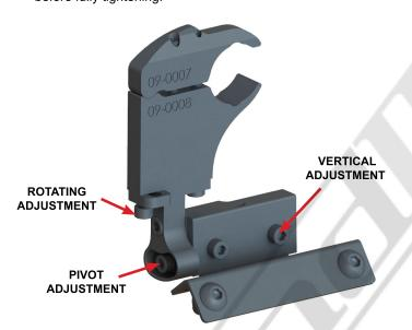
Reinstall the body assembly. Be sure to include all lock washers with screws, and the lock and flat washer with the bottom socket head screw. Use the adjustments shown above to adjust the RD to you.
